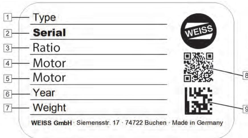
Figure 1: Example of nameplate
