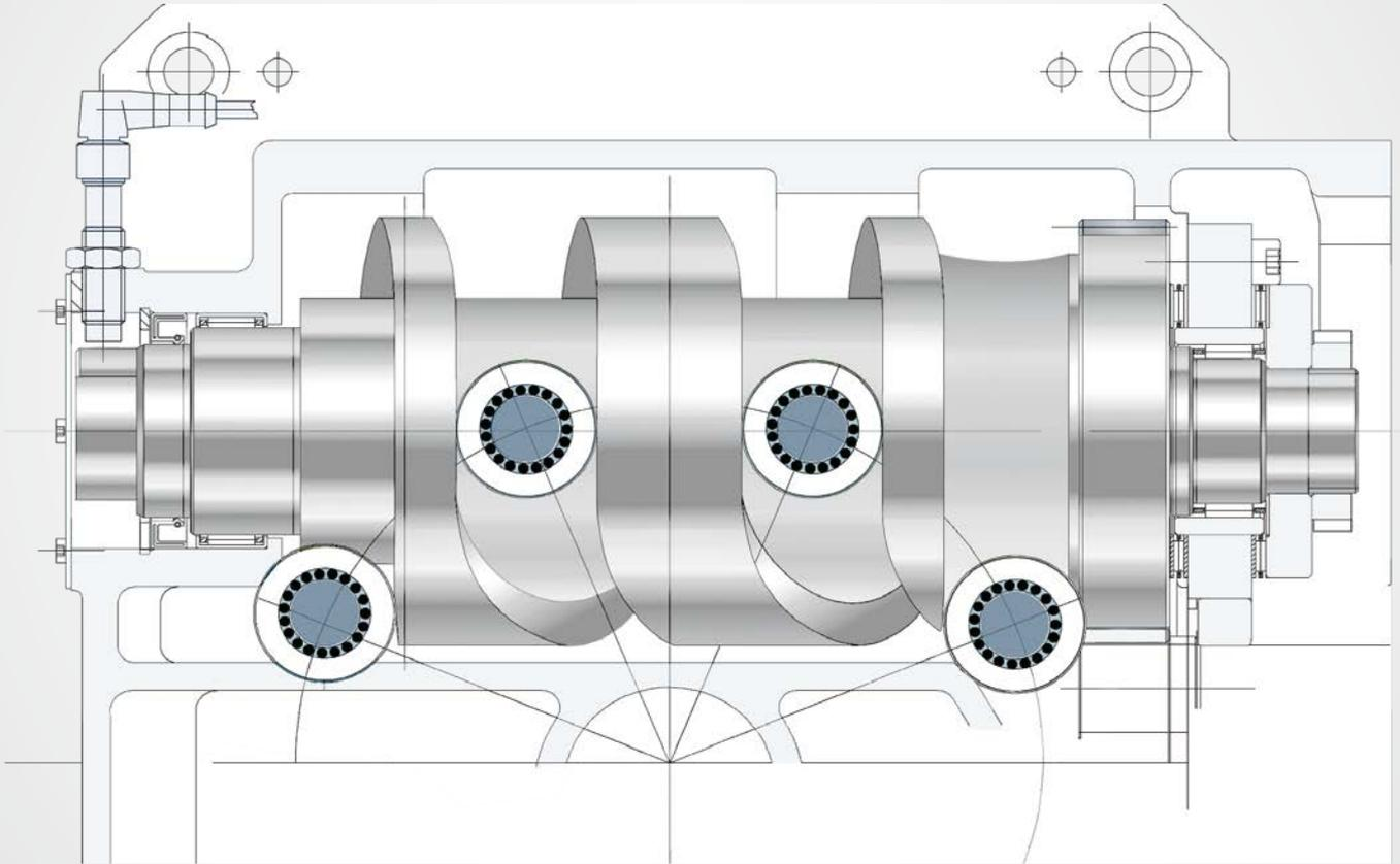
The TC is one of the most reliable and robust rotary indexing tables available worldwide. Our roller cam drives are dimensioned as large as possible. And the full length of the cams is used here.
