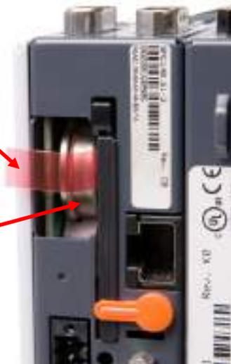
5. Push the end of the pullout strip that stands out under the battery, so that it does not extend from the battery compartment.
