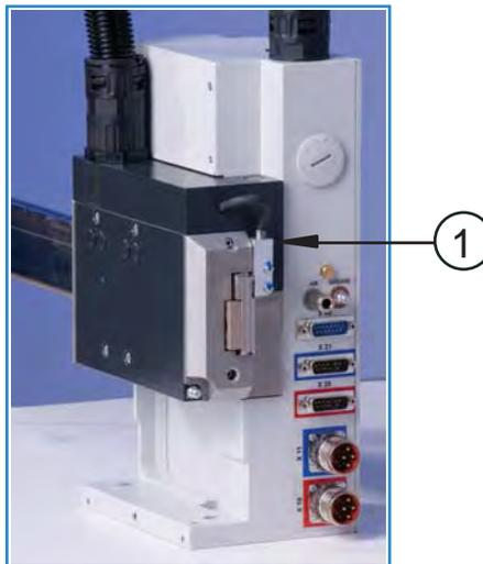
**Fig. 20: Lubricating spring**
