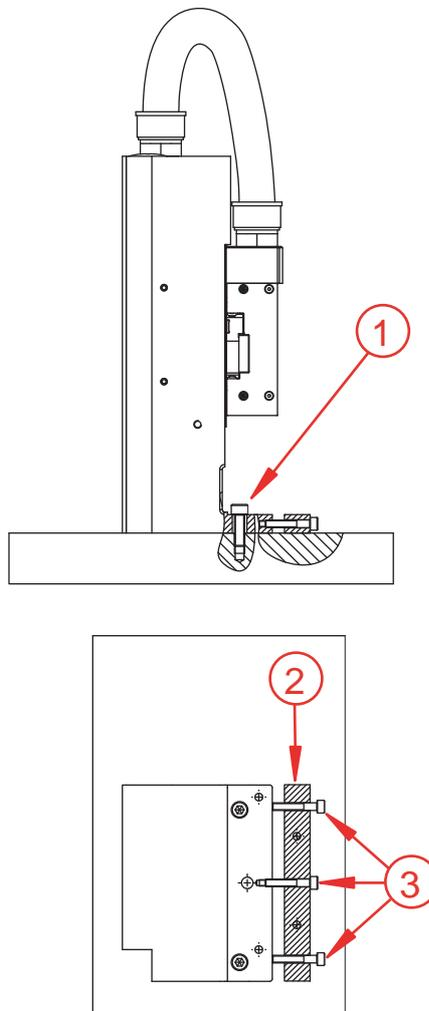
Fig. 14: Adjustment via long holes
