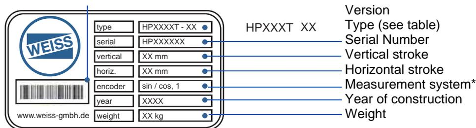
\* sinus / cosinus measurement system with pole pitch of 1 mm
