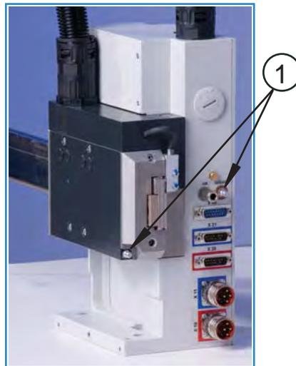
Fig. 10: Connections for automatic lubrication
