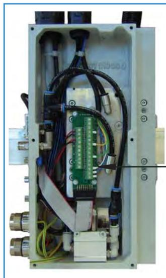
A board with terminals for applying digital inputs and outputs can be found inside the housing.
