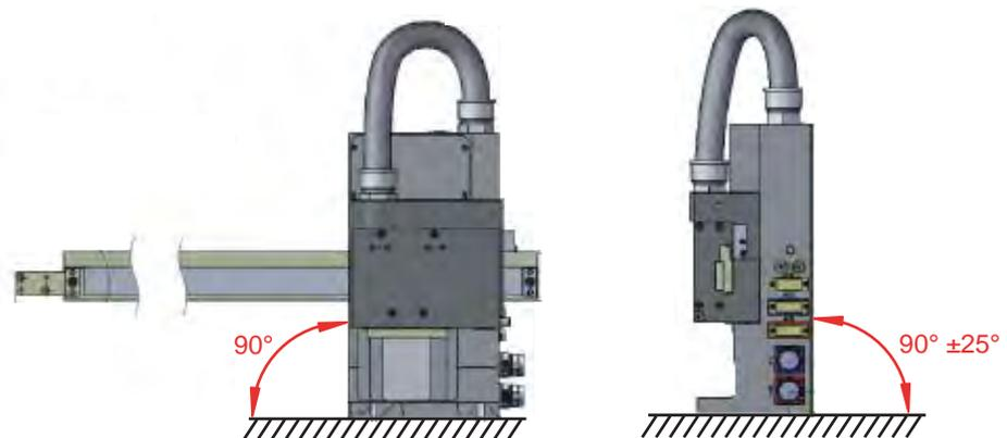
Fig. 4: Installation positions
